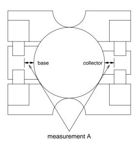
Figure 5.2 Typical Transistor/Capacitor Spacing (Not To Scale)
