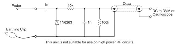
unit is not suitable for use on high power it. Circuits
